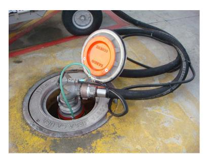
Hydrant coupler and aircraft fueling nozzle swivel retention devices must be equipped with at least two levels of redundancy, such as collar lock rings and collar retention screws secured by safety wire.
